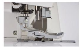
Adjustable Presser Foot Height up to 6mm Accolade features a higher presser foot height to effortlessly handle thicker and loftier fabric.
