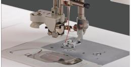
Advanced Needle Threader Threading a needle has never been easier than with this innovative threader. With just a few simple motions, your needle is threaded and ready to use it's so easy, you can do it with one hand!
